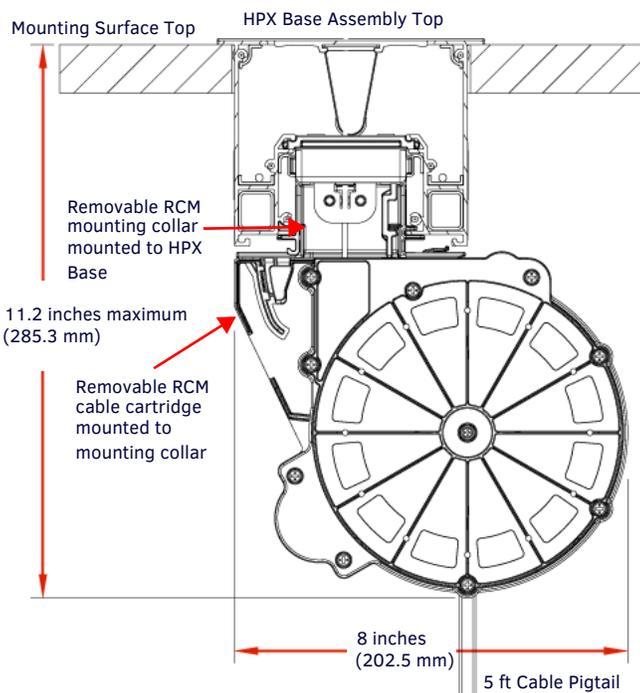
FIG. 6 RCM MODULE (INSTALLED IN AN HPX BASE) - DETAILED DIMENSIONS
