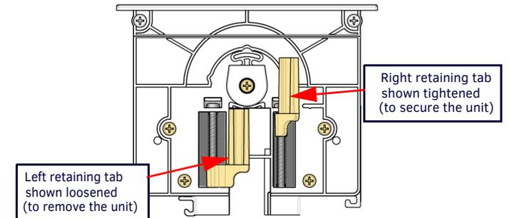
FIG. 9 HPX BASE ASSEMBLY (SHOWN MOUNTED) - MOUNTING SCREWS LOCATIONS
