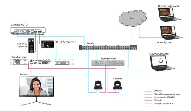
> The Plixus Gateway can be connected either to the WAN port, the LAN port or both. In case both the WAN and LAN ports are used, two switches and two DHCP servers will be necessary.
