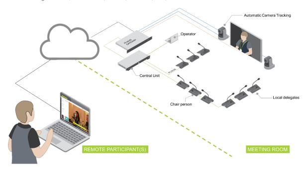
Figure 1-1 Typical Plixus Gateway setup where the gateway is connected to the Cloud, the Central Unit, the screen and the cameras
