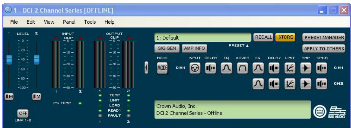
Figure 17 With the "Y 1+2" box checked, both output Ch.1 and Ch.2 are fed by input Ch.1 and input processing is organized accordingly.
